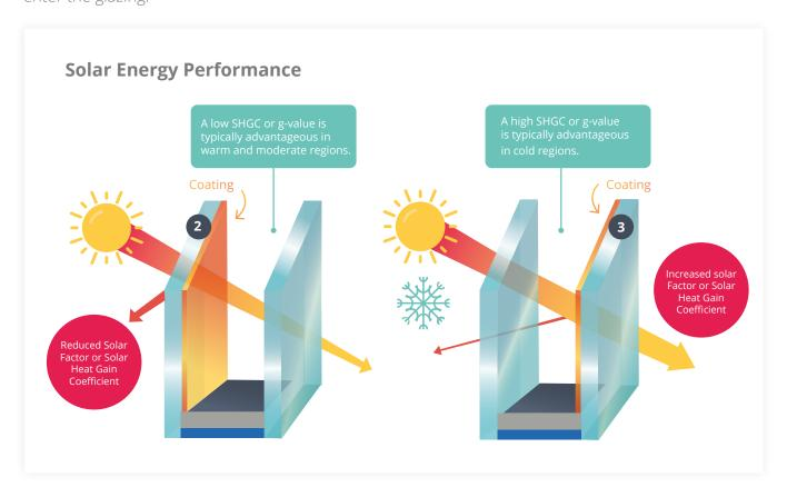
Light coming inside the building, as well as coatings and their placement in the glazing, are crucial in **supporting occupant comfort**. The term '**spectral selectivity**' is used to address the amount of daylight transmission relative to solar energy blockage. Greater spectral selectivity is achieved when more visible light, and less overall solar energy, is transmitted.
