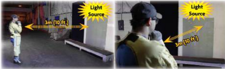
Image 19 – Visual Inspection of transmission (light source behind glass)
