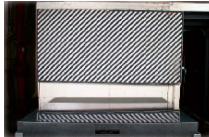
Image 32 – Zebra board mounted off-line
