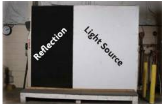
Image 18 – Solid backgrounds to simulate outdoor reflected color (Black) and transmission color (White)
