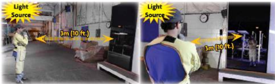
Image 20 – Visual Inspection of reflection (light source behind or above inspector)
