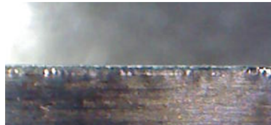
Image 22 – Glass cut at the same cutting wheel angle, speed, and head pressure as in Image 21, but with poor score depth.
