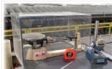
Image 38 – Tape measure, scale and feeler gauge
