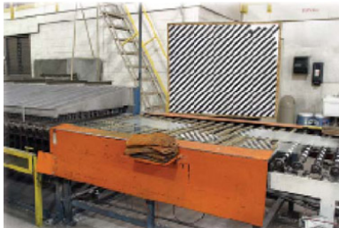
Image 31 – Zebra board mounted on-line
