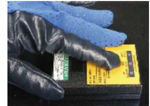
Image 14 – Low-E surface detector
